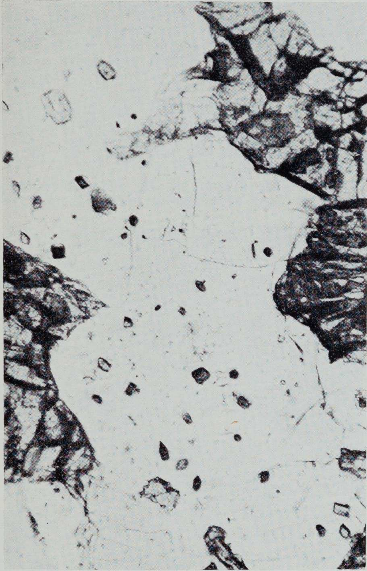
Figure 2.—A (left) Photomicrograph of a plagioclase grain (white) in Spec. 16311 showing euhedral spinel inclusions (shades of dark grey). The other dark mineral is clinopyroxene which contains some vermiform spinel inclusions. Plain light, X80. B (right).—Same field of view as Figure 2A with nicols crossed. Note the andesine haloes around spinel inclusions in the labradorite host.
